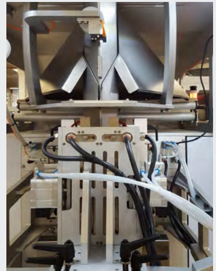
Vertical sealing and forming tube details
