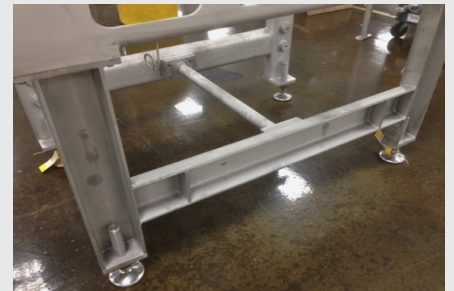
Open Channel Frame with no hollow tubing and no flat level surfaces
