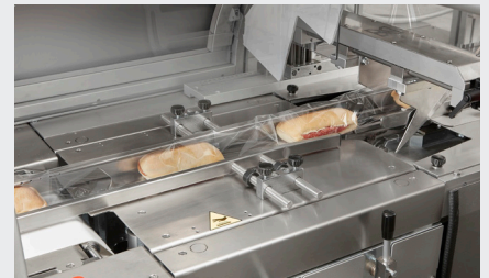
Longitudinal Sealing Station
